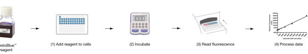
Figure 21— Workflow of the PrestoBlue™ Cell Viability Reagent. The PrestoBlue™ Cell Viability Reagent comes as a ready to use 10X Solution. Simply add the PrestoBlue™ reagent to cells, incubate for as little as 10 minutes, read the fluorescence (or absorbance), and process the data.
